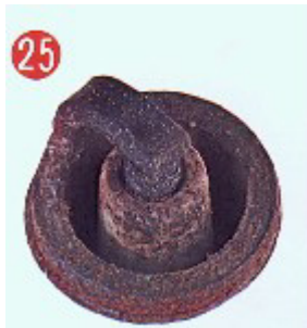
25 Too Hot or Lean Pre-Ignition Range
